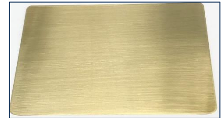
Sanded Hull-Cell panel Grain size 800
