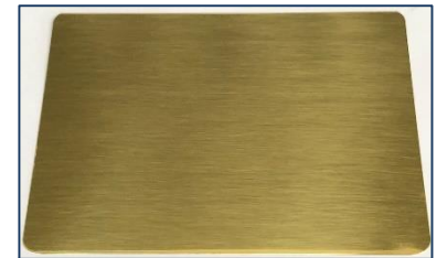
Fully bright polished Hull-Cell panel
